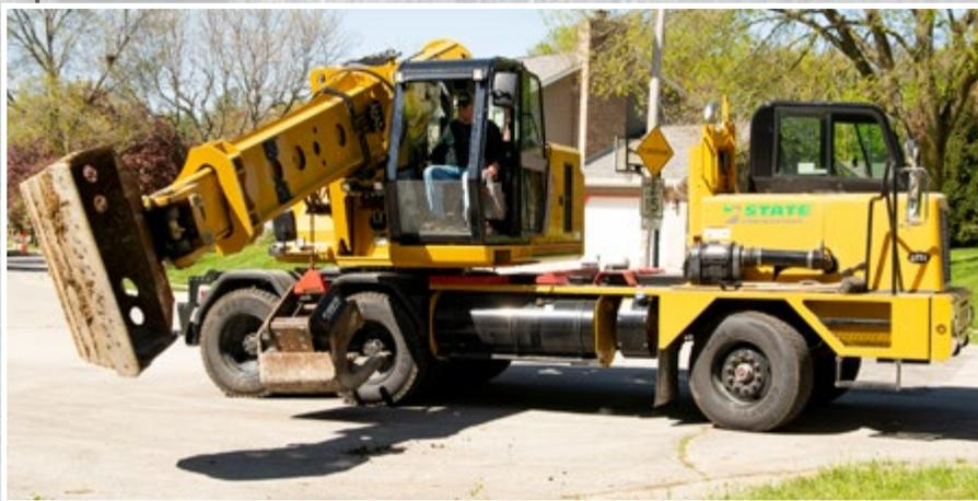
tilting, telescoping boom. Then, without assistance, he can easily change to the pavement removal bucket for pulling sections of curbs, gutters and sidewalks, reaching under trees and handling slopes
