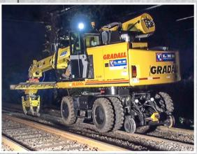
machine and uses the rubber tire undercarriage for mobility. To address rail tie deterioration, the XL 3300V operator uses a Rosenquist SB60 attachment and the excavator's full-tilting boom movements to carefully extract and replace the ties, and then evenly spread ballast. Improper drainage can make track unstable and maintenance more intensive, so a Gradall is frequently used to clear ditches or replace culverts. Other times, buckets are used to rebuild
