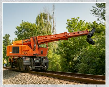
also is operated from ground level as it deploys onto the track with an articulated dual-scissor action. This mechanism provides a "side-shift" action, making it easier for operators to align the Gradall machine to the track.
