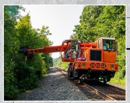
From the equipment yard to the crossing, where the XL 4130 V is mounted on the track, mobility is exceptional at speeds up to 60 miles per hour, driven from the chassis cab. On track, the machine is
