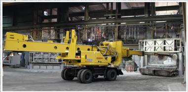
requirements. • "We are using the Gradall to skim dross from two furnaces," added Tabor, "while we work with Gradall to design another machine with an even smaller footprint to work in tighter confines."
