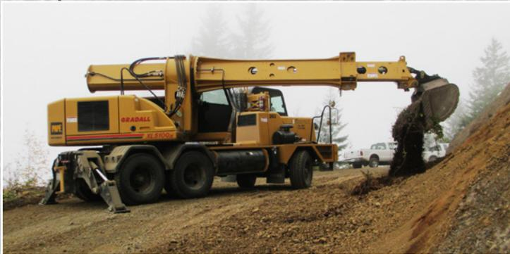
including the ability to reposition the machine from the upperstructure operator cab. “The remote drive is important, especially on hilly terrain,” he said. ❖ Meier also appreciates the full-boom tilt capability and extra boom reinforcement on the Series IV model to create more boom strength.
